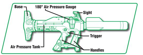
Place your feet on the Base, and use the Handles to Pump the missile blaster approximately 16 times.
