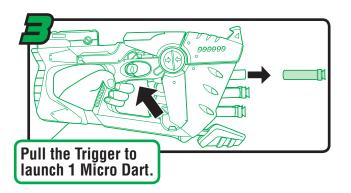
NOTE: You must slide the Multi Shot Mechanism forward and back to its original position before pumping the dart blaster. Otherwise, only one dart will launch and blast mode will not function properly.
